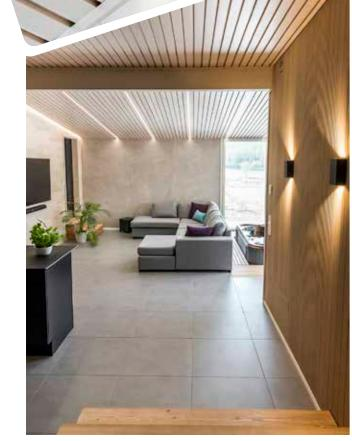
The VALO panelling has been designed for use on ceilings. The design gives a slatted effect but is quick to install thanks to the finished edges. The panels are quick to slot together and, unlike with traditional slatted finishes, you won't need to worry about ensuring that the surface behind them flawless.
