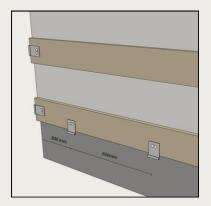
When the cladding panels are installed vertically, the furring strips are fastened crosswise. First fasten the vertical studding, and then nail the furring strips on top of the studding max. 600 mm apart. The cladding panels are fastened on top of the crosswise studding. If the furring strips are fastened more than 600 mm apart, design the structure again.
