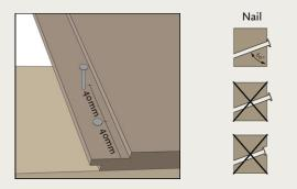
Drive the nails at about 60° degree angle to ensure that the tongue is not damaged while fastened. Fasten the panels tightly against one another. Make sure that the tongues are pressed all the way to the bottom. Check regularly with a spirit level that the cladding panels are straight.
